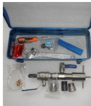
Hot taping driller
