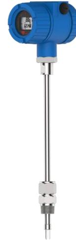
The In-line type is delivered along with a pipe which has a same inner diameter as the pipe in field. It should be installed through flange or screw thread. The flanges meet GB/T9119-2000 standard (or ANSI B16.5 or DIN or JIS standard). The in-line type can fit in pipe with diameter from DN15mm to DN300mm. Or customer can simply choose to use a 3-way pipe to replace the flanged body
